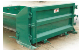
Watertight containment minimizes the risk of caustic wastewater being disposed of improperly.
