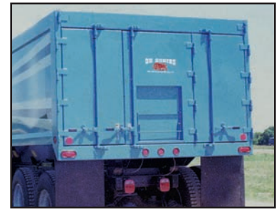
Standard 3-door rear gate with center grain chute.
