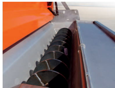
Fully tapered trough eliminates all flat surfaces preventing material hang ups.
