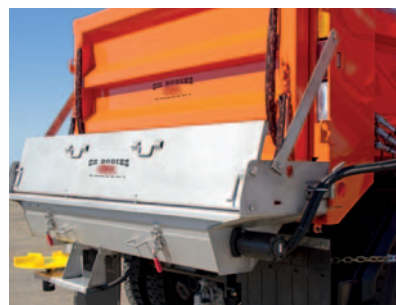
Direct drive design minimizes maintenance and allows independent control of auger and spinner.
