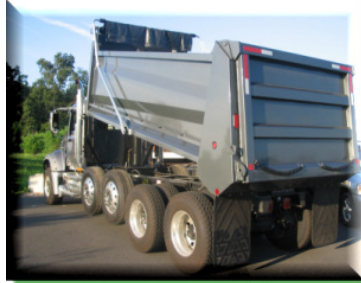
Full depth rear corner post for stability and durability
