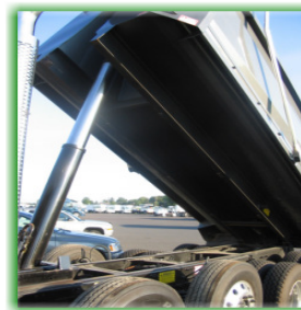
Continuous welds minimize moisture build up, preventing rust
