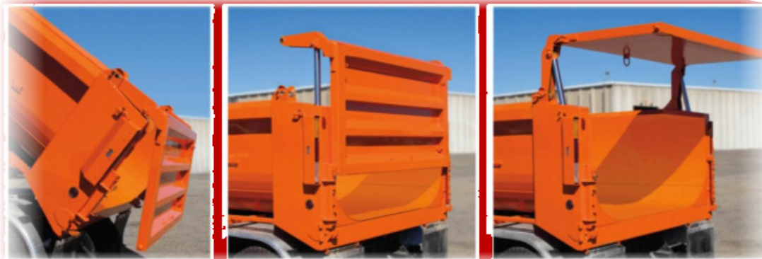
High Lift and Sliding Tailgate "all-in-one" option for 5 yard bodies and larger. You can't find it anywhere else.
