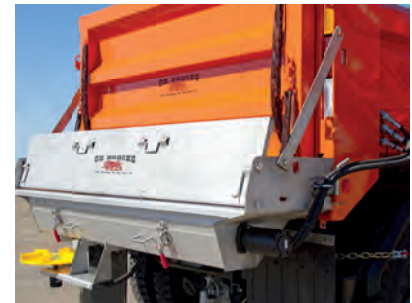
Direct drive design minimizes maintenance and allows independent control of auger and spinner.
