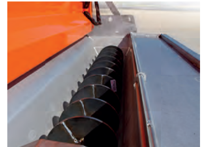
Fully tapered trough eliminates all flat surfaces preventing material hang ups.
