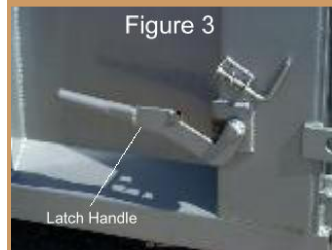
Figure 3. Unlock top latch with handle as illustrated. Note: Never unlock this mechanism without first inserting pin with safety pin as seen in figure 1.
